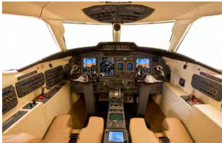
The Sino Swearingen SJ30 cockpit features the Honeywell Primus Epic™(CDS) avionics package.
